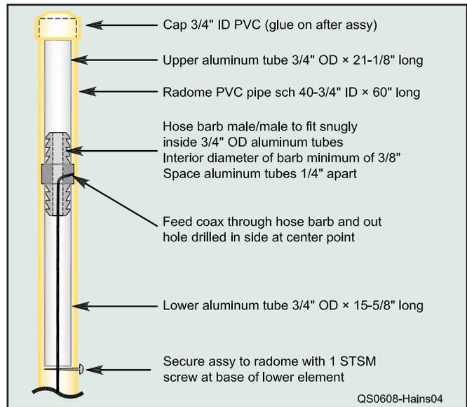
Figure 4 — Details of antenna installation in radome.
